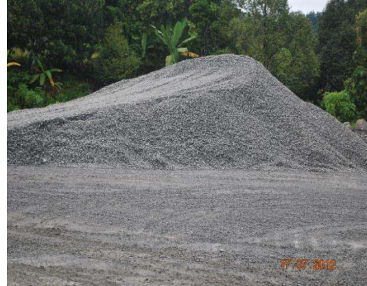
Gambar 3.22 Stockpile- Batu Aggregate
